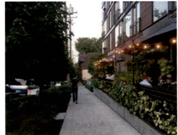
Set buildings back from the property line to allow for more pedestrian level outdoor space.
